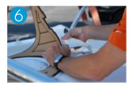
Once the piece is in place and backing paper fully removed press down on the entire surface to ensure bond.
