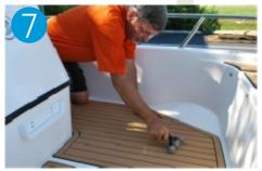
Continue with the rest of the areas to be covered with mats using the same method, and ensuring alignment of each piece before sticking them down.
