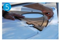
Align the first piece to be installed and hold in place - tape it down if the piece is large with a few pieces of masking tape. It is a good idea to have the next piece with you while aligning this piece to ensure proper alignment. Once you have the piece aligned and taped in place you should lift one side about half way back and begin peeling the backing paper from the cut you made earlier. Let the piece slowly roll down into position being careful not to tug or distort its shape.
