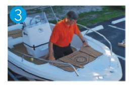
Lay all pieces into their proper area for installation and check for fit and alignment. Once you are happy with the fit it is time to install. We suggest beginning at either the front or back and working towards the other direction.
