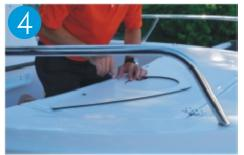
Score the backing paper on the first piece to be installed in the middle of the mat using your razor knife. Be careful not to cut too deep.
