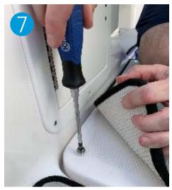
Using the screwdriver, tighten the snap stud through the washer the washer in the hole and snap the mat in.
